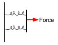
The force exerted on the spring combination is equal to the sum of the forces exerted on each spring
